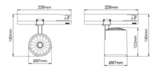
**SPECIFICATIONS** Lightsource Type: LED (built in) System Power [W]: 30W CCT (Color Temperature): 4000K CRI / Ra: 90 Lumen Output: 4236lm Lumen LED (tc=25): 4250lm Beam Angle: 30° Lens (Diffuser): Clear Dimming: DALI2 System Voltage [V]: 230V 50Hz Connection: Track 3-Circuit+dim Mounting: Track, Ceiling Lifetime [h]: L80B10: 100 000h Lumen/W: 141lm/W MacAdam (SDCM): 3 Color: Black Length [mm]: 260mm Height [mm]: 180mm Width [mm]: 97mm Weight [kg]: 0,841kg
