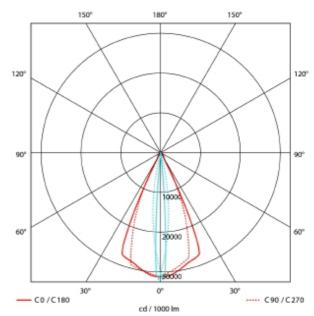
Zoom Mini is relatively small spotlight for use in track lighting systems. The unique zoom patent makes it possible to vary the beam angel between 5 - and 60 degrees making this model highly versatile. This Zoom Mini version comes with 2700 Kelvin and DALI2 driver. It's made from robust die-cast aluminum.
