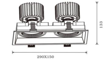
Quadro, a new downlight available in a single and a double version. The Quadro combines the design details from track mounted spotlights with those of downlights. This will make a very nice design element in premises where one needs both track mounted and recessed fixtures.
