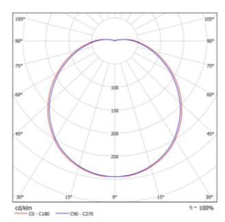
Surface mounted LED plafond with direct light distribution. Opal PMMA diffuser and steel housing. UGR index: =22. IP44. IK02. 3 hours emergency with Selftest.
