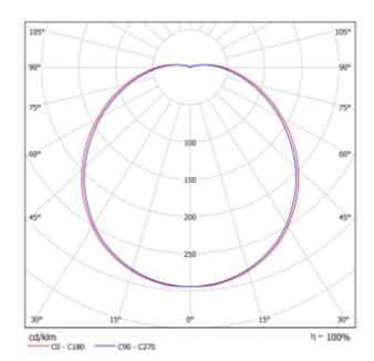
Surface mounted LED plafond with direct light distribution. Opal PMMA diffuser and steel housing. UGR index: =22. IP44. IK02. Options: microwave (master) sensor, Master-Slave by RF (wireless), emergency function and more.
