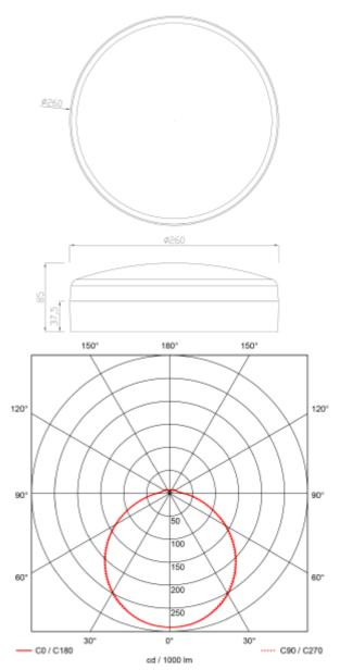
Caph is as surface mounted ceiling light with opal diffuser and microwave motion and daylight sensor.
