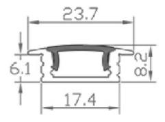
Anodized Aluminum profile for recessed mounting.
