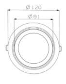
Our Trimo range of downlights guarantees a minimum of stray light. This is accomplished by using a recessed LED light source. This model requires a hole dimension of 112mm in diameter making it very versatile providing very powerful light. The Trimo Mini has a 18i3 connector and is supplied with a variety of connector solutions.
