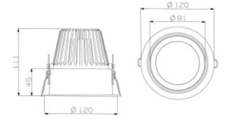
**SPECIFICATIONS** Lightsource Type: LED (built in) System Power [W]: 24W CCT (Color Temperature): 3000K CRI / Ra: 80 Lumen Output: 2890lm Lumen LED (tc=25): 3650lm Beam Angle: 40° Lens (Diffuser): Clear Dimming: DALI System Voltage [V]: 230V 50Hz Connection: 18i5 DALI Quick connection
