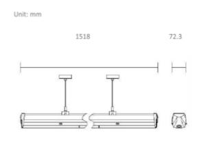
**( €** ☐ IP20 | 230V | 50Hz | **SPECIFICATIONS** Lightsource Type: LED (built in) System Power [W]: 70W CCT (Color Temperature): 3000K CRI / Ra: 80 Lumen Output: 10800lm Lumen LED (tc=25): 11000lm Beam Angle: 60 Lens (Diffuser): Clear Dimming: None Flickerfree: Yes System Voltage [V]: 230V 50Hz Connection: Trunk 8-wires Mounting: Suspended, Ceiling Lifetime [h]: L80B10: 100 000h Lumen/W: 154lm/W Color: White Length [mm]: 1500mm Height [mm]: 78,6mm Width [mm]: 72,3mm Weight [kg]: 1,67kg
