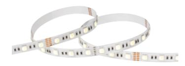
LED-strip of high quality. Available in 2700K or 3000K. For outdoor mounting og mounting in bathrooms, a IP65 version is available. CRI95 secures correct color reproduction, which is important for lighting over mirrors on bathrooms for example. Length is 5 meters, with 19,2W/m. For best looking and cooling the LED-strip we recommend mounting in aluminium profile. See accessories for recommended drivers.
