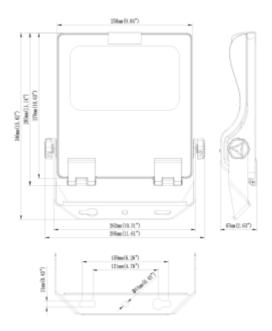
lota G2 is a highly cost-effective floodlight that comes with a power switch in various sizes, equipped with front clips for easy access to the dip switch. It is equipped with asymmetric optics that make it ideal for a variety of applications. For post mounting, a mounting bracket can be purchased separately. With a solid IP rating of IP66, it is perfect for outdoor use in various environments.
