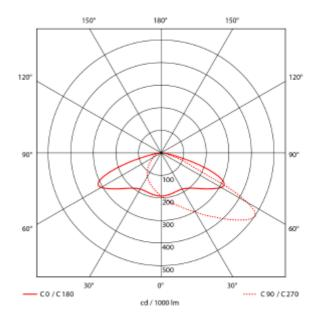
Coxa is a top quality LED wall pack designed for outdoor areas lighting and courtyard illumination. With Asymmetrical light distribution, Coxa is good to replace 250W Metal Halide lamps. With powder coating and sand textured housing, Coxa has good performance of corrosion-resistance. Defalt setting 70W. By using dip-switchit can be 53W/35W or 21W. 21W = 3200lm 35W = 5130lm 53W = 7685lm 70W = 9850lm
