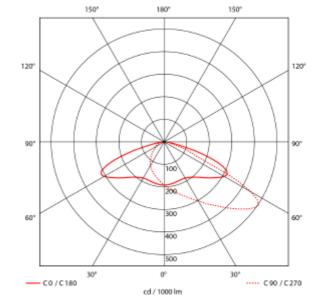
Coxa is a top quality LED wall pack designed for outdoor areas lighting and courtyard illumination. With Asymmetrical light distribution, Coxa is good to replace 250W Metal Halide lamps. With powder coating and sand textured housing, Coxa has good performance of corrosion-resistance. Defalt setting 70W. By using dip-switchit can be 53W/35W or 21W. 21W = 3260Im 35W = 5245Im 53W = 7890Im 70W = 10050Im
