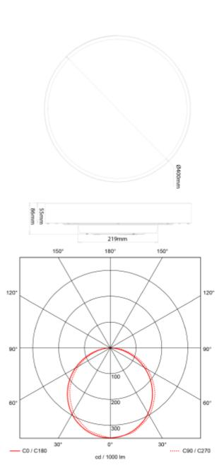
Galactic C is our new series of circular lamps. Modern design combined with prismatic diffuser that gives a pleasant and comfortable light. Galactic has several mounting options, recessed, semi-recessed, surface mounted or suspended. Choose between 2700K and 3000K (dip-switch) with dircet light or direct / indirect light. Galactic is delivered in size: Ø400mm, Ø600mm, Ø800mm and 1000mm.
