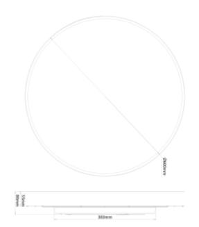
Galactic C is our new series of circular lamps. Modern design combined with prismatic diffuser that gives a pleasant and comfortable light. Galactic has several mounting options, recessed, semi-recessed, surface mounted or suspended. Choose between 2700K and 3000K (dip-switch) with dircet light or direct / indirect light. Galactic is delivered in size: Ø400mm, Ø600mm, Ø800mm and 1000mm.
