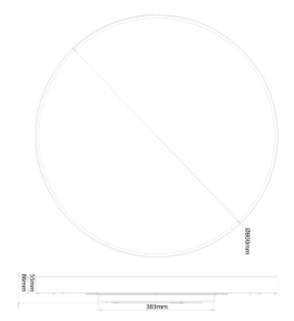
Galactic C is our new series of circular lamps. Modern design combined with prismatic diffuser that gives a pleasant and comfortable light. Galactic has several mounting options, recessed, semi-recessed, surface mounted or suspended. Choose between 2700K and 3000K (dip-switch) with dircet light or direct / indirect light. Galactic is delivered in size: Ø400mm, Ø600mm, Ø800mm and 1000mm.
