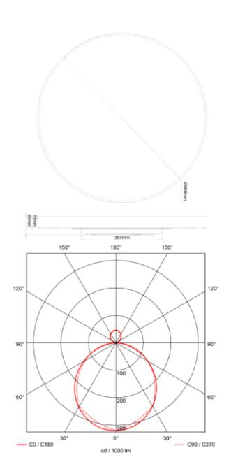
Galactic C is our new series of circular lamps. Modern design combined with prismatic diffuser that gives a pleasant and comfortable light. Galactic has several mounting options, recessed, semi-recessed, surface mounted or suspended. Choose between 2700K and 3000K (dip-switch) with dircet light or direct / indirect light. Galactic is delivered in size: Ø400mm, Ø600mm, Ø800mm and 1000mm
