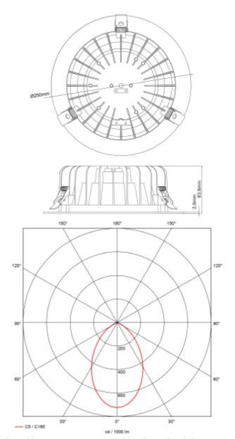
Leila R with cut out Ø240mm. Developed to change from halogen to downlight with latest LED technology. High Efficiency, easy installation. Delivered without driver. See accessories for correct driver-
