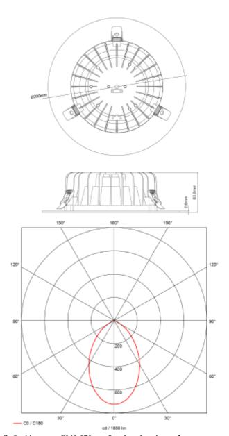
Leila R with cut out Ø240-270mm. Developed to change from halogen to downlight with latest LED technology. High Efficiency, easy installation. Delivered without driver. See accessories for correct driver-
