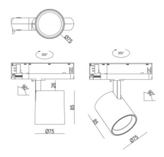
Rod Mini C is perfect for illuminating small areas such as walkways, stairs, or shelves to create a cozy atmosphere. With an impressive color rendering index (CRI) of over 80 and a warm color temperature of 3000K, Rod Mini C provides pleasant and atmospheric lighting with a light output of 350 lm/m and an efficiency of 80 lm/W. The product has a diameter of 75 mm, height of 85 mm, and an IP rating of IP20, making it suitable for indoor use.
