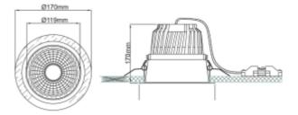
Tired of downlights giving obtrusive annoying stray light? Our Trimo range of downlights guarantees a minimum of stray light, this is accomplished by using a recessed LED light source. The Trimo range has a 18i3 connector and can be supplied with a variety of connector solutions.
