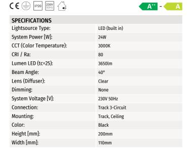
Ray Mini uses the possibillities created by new technology. The LED driver is mounted inside the luminare body. This gives us a slim design combined with a powerful lightoutput that can be easily adjusted in all directions to meet all needs. Ray Mini can be tilted 90 degrees and rotated 350 degrees its own axis. To create further opportunities to play with light you can mount a diffuser on the luminaire, this can be ordered separately.
