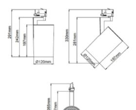
Ray Maxi, a powerful spotlight in the Ray family using a design concept with the LED driver built in to the spotlight body. This gives a modern, slim design with a high lumen output. The Ray Maxi can be tilted 90 degrees and rotated 350 degrees on its own axis offering create flexibility in playing with light. A diffuser can be mounted on the luminaire, to be ordered separately.
