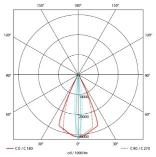
Zoom Mini is relatively small spotlight for use in track lighting systems. The unique zoom patent makes it possible to vary the beam angel between 5 - and 60 degrees making this model highly versatile. This Zoom Mini variant is available in both black and white color, 2700 and 3000 Kelvin and with phase cut dimming. The spotlight is made from robust die-cast aluminum.
