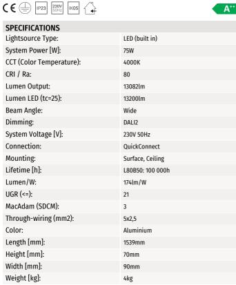
Bladeline Z is a highly efficient LED luminare with up to 179lm/w. Due to fact that it may be installed surface mounted on the ceiling or on electrical tracks makes it highly flexible. Can be opened without using tools and it has the electric connectors on quick fit clamps. The Bladeline Z is made from galvanized steel with medium or wide beam (75° and 90°) optic in 42W or 75W versions.
