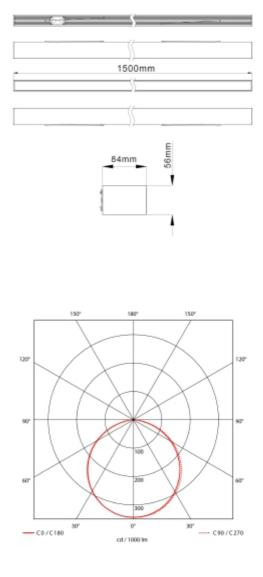
LEDline is a modern linear LED system for seamless lighting. It is based on modular chassis details allowing for seamless extensions through both straight connectors, 90 degrees corners and X-crosses. This allows light designers to make tailor fit lighting systems in an easy manner. The chassis details assure easy installation without failures. Add 1 pc 8050-05 for each mains supply (each row or standalone). Also add mounting accessories.
