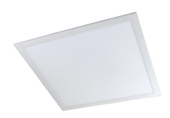
Panel LED is a light fixture for interior use. It is constructed for fitting in to suspended ceilings. Panel LEDs can be installed as a pendant or mounted on ceiling surfaces. The Panel LED has an opal or micro prismatic diffusor. Choose between ON/OFF, Phase-Cut or DALI2 (CLO, Corridor, Push dim and Ready2mains) driver. See accessories for detailed information.
