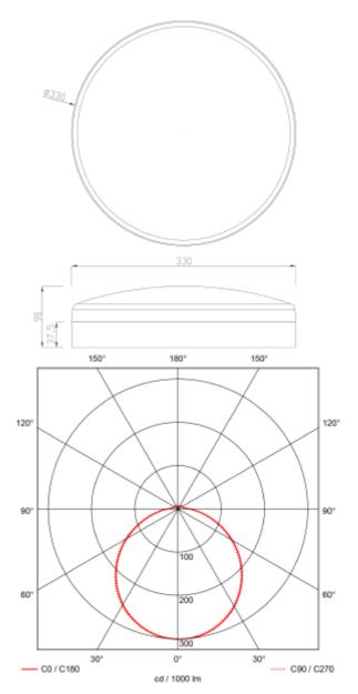
Caph is as surface mounted ceiling light with opal diffuser. Comes with a switch option between 3000K(default), 4000K and 5700K. Quickconnect for easy installation.
