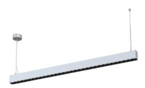
The Phoenix is a linear LED luminaire with up- and down light for pending down in indoor areas. The light distribution is 2000 lumen upwards with a 140° reflector and 2000 lumens downwards with a 80° reflector. It is made from durable aluminium for easy care. The color temperature is 3000 Kelvin and the reflectors secures a pleasant light. 3m wire.
