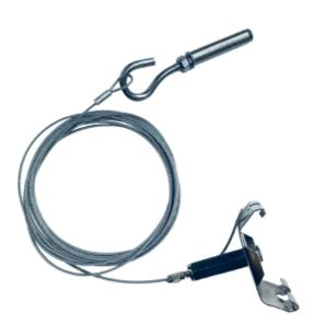
Wirekit 3m for Trunk. First clip attachment point starts at 100-800mm. Recommended distance between mounting bracket are maximum 2000mm. Are distance 2m between each bracket, are total brackets needed: length of track dived by 2 + 1 pcs. Diameter of hole in concrete are Ø10mm. Control correct diameter before you start.
