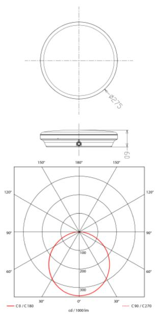
Dimmable surface mounted ceiling light with PC diffuser and even light output. IP54 waterproof structural design, its an ideal replacement for wet locations. Comes with a switch option between 2700K(default)and 3000K. Dimmable by phasecut or DALI2. QuickConnect for easy installation.
