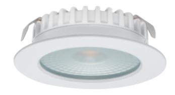
This furniture downlights makes it very easy to replace from old halogen fittings with LED technology. Integrated push-in terminals enable to use existing dimmer, transformer and wires. Replaces halogen downlights with hole measurements 57-60mm. Connect to 12V AC/DC, and can be dimmed on AC.
