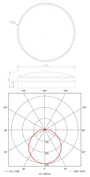
Caph is as surface mounted ceiling light with opal diffuser and microwave motion and daylight sensor.
