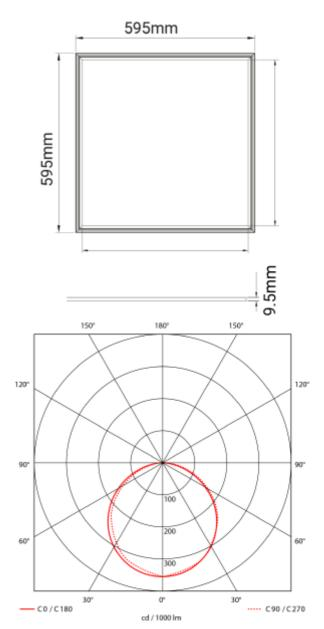
Panel LED is a light fixture for interior use. It is constructed for fitting in to suspended ceilings. Panel LEDs can be installed as a pendant or mounted on ceiling surfaces. The Panel LED has an opal or micro prismatic diffusor. Choose between ON/OFF, Phase-Cut or DAL12 (CLO, Corridor, Push dim and Ready2mains) driver. See accessories for detailed information.
