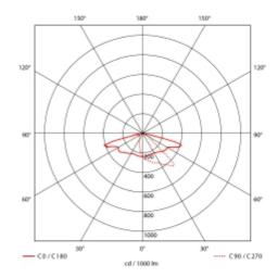
Via is a luminaire for post mounting. We have developed this luminaire with an asymmetrical reflector giving a wide spread light, see light distribution diagram below. Via has a post fixation opening with a diameter of 60mm. The luminaire has an IP66 classification and this guarantees that it will withstand very demanding conditions.
