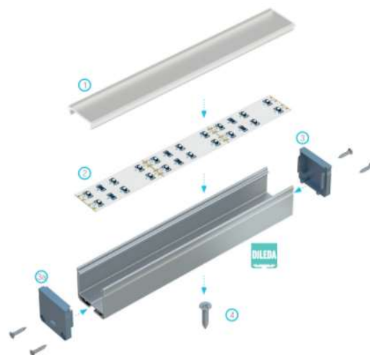
Assembly scheme for elements of the lighting system using profile DILEDA and (1) DOUBLE cover (2), LED strips, (3) end cap without hole, (3a) end cap with hole and (4) mounting screw
