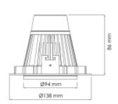
A\*\* -**SPECIFICATIONS** Lightsource Type: LED (replaceable) System Power [W]: 35W
