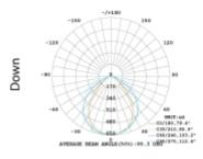
Office slim is an elegant and slim luminaire to use in all offices. Light distribution: 70% down & 30% up. Turn on/ off by hand movement. Complete with canle and 1500mm wire.
