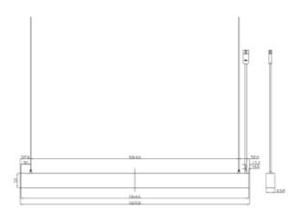
Benu is a linear LED luminaire with up- and down light for pending down in indoor areas. UGR19 and DALI2. 18i5 connection, 1500mm transparent wire and T-profile bracket are included.
