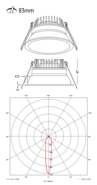
Ceto Mini fixed is a low downlight with 7W effect. With recessed light source, low blending, CRI95 and 18° beam angle, this is the natural choice where you want to create an exclusive and comfortable lighting. Phase-cut driver included.
