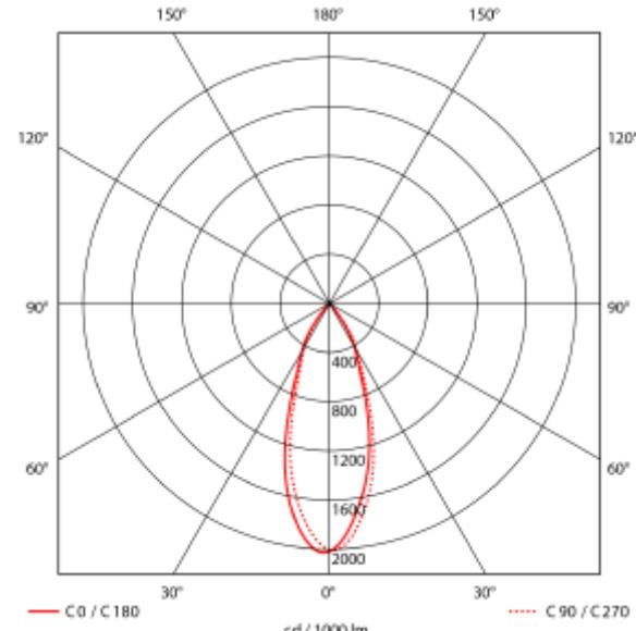
Phoenix Downlight has the latest LED technology, with micro reflector and anti-glare cover it reaches UGR17. With 35° beam angle and perfect light cutoff it's the ideal downlight for office, hotel, staircase, and corridors. Delivered with out driver, see accessories to find suitable driver.
