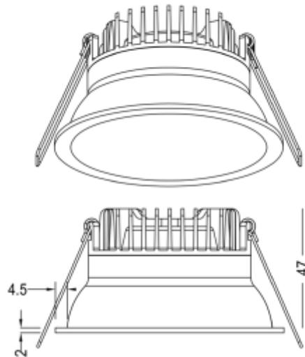
Ceto Mini fixed is a low downlight with 7W effect. With recessed light source, low blending, CRI95 and 36° beam angle, this is the natural choice where you want to create an exclusive and comfortable lighting. Phase-cut driver included.
