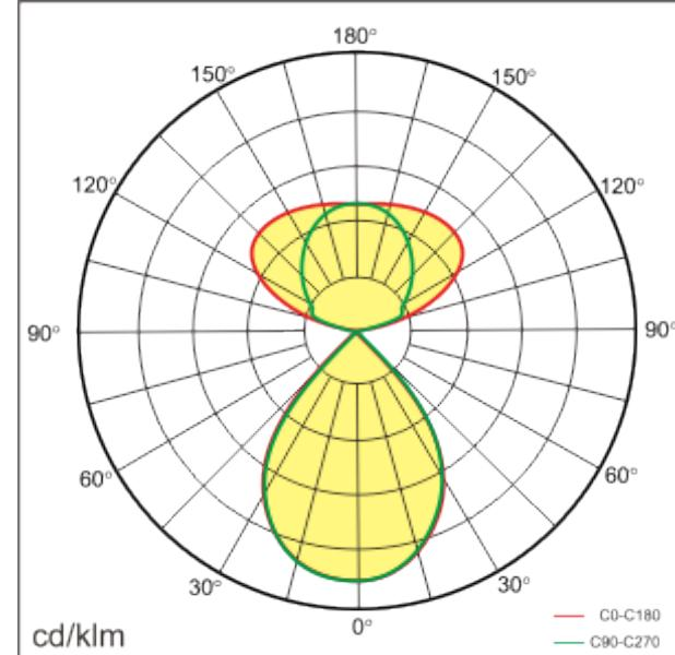
The Phoenix is a linear LED luminaire with up- and down light for pendant down in indoor areas. The light distribution is 2000 lumen upwards with a 140° reflector and 2000 lumens downwards with a 80° reflector. It is made from durable aluminium for easy care. The color temperature is 3000 Kelvin and the reflectors secures a pleasant light. 3m wire.
