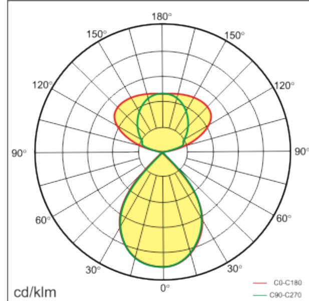
The Phoenix is a linear LED luminaire with up- and down light for pending down in indoor areas. The light distribution is 2000 lumen upwards with a 140° reflector and 2000 lumens downwards with a 80° reflector. It is made from durable aluminium for easy care. The color temperature is 3000 Kelvin and the reflectors secures a pleasant light. 3m wire.
