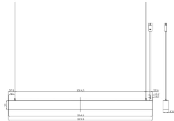
Benu is a linear LED luminaire with up- and down light for pending down in indoor areas. UGR19 and DALI2. 18i5 connection, 1500mm transparent wire and T-profile bracket are included.
